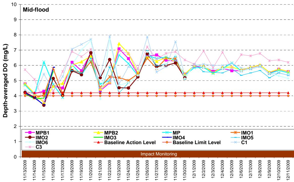
Figure F1 Dissolved oxygen concentration (depth-averaged) (mg/L) of water samples at mid-ebb and mid-flood between 13 November and 11 December 2009
