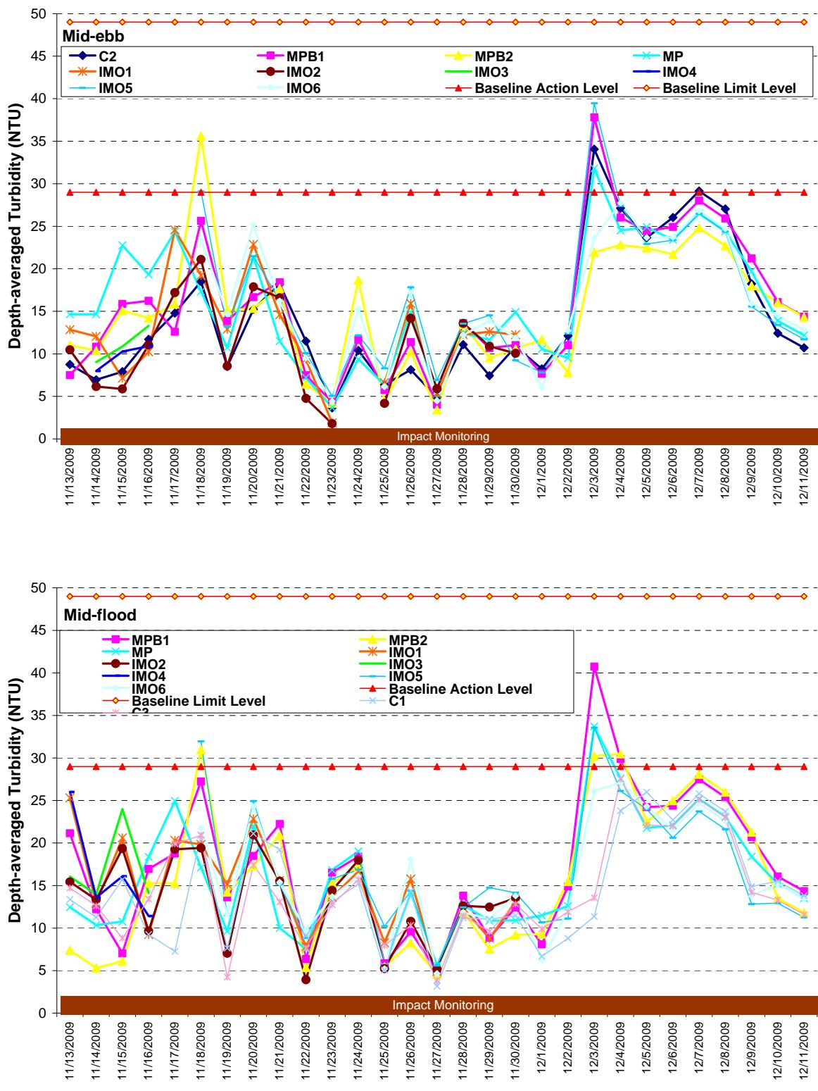
Figure F3 Depth-averaged turbidity (NTU) of water samples at mid-ebb and mid-flood between 13 November and 11 December 2009
