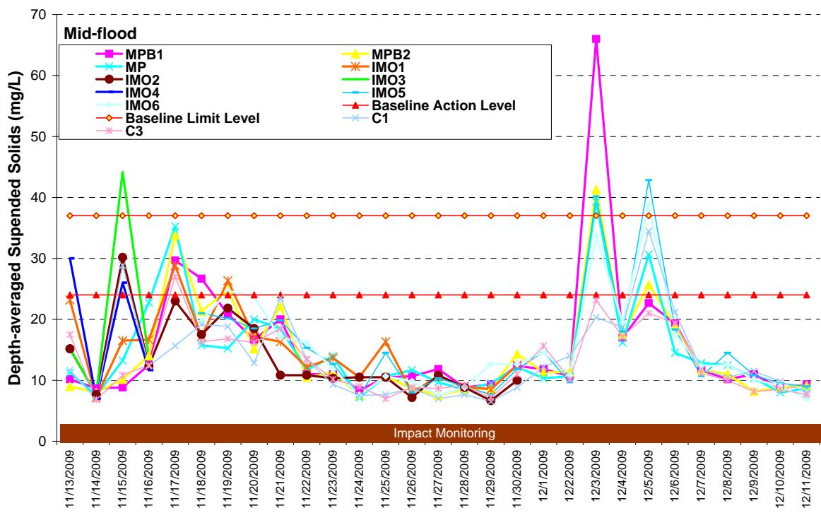
Figure F4 Depth-averaged suspended solids concentration (mg/L) of water samples at mid-ebb and mid-flood between 13 November and 11 December 2009
