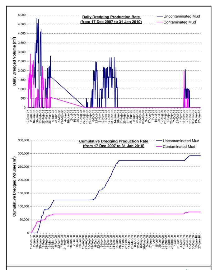
Figure 2.1 Daily and cumulative volumes (m³) of excavated materials (both contaminated and uncontaminated mud) from 19 December 2007 to 31 January 2010.
