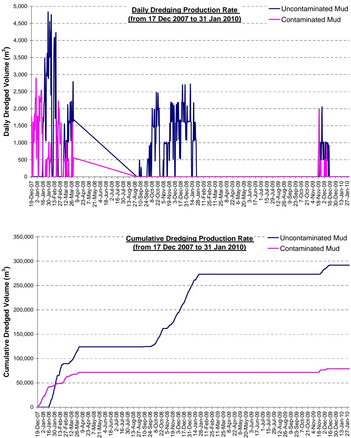
Figure 2.1 Daily and cumulative volumes ( $m^3$ ) of excavated materials (both contaminated and uncontaminated mud) from 19 December 2007 to 31 January 2010.
